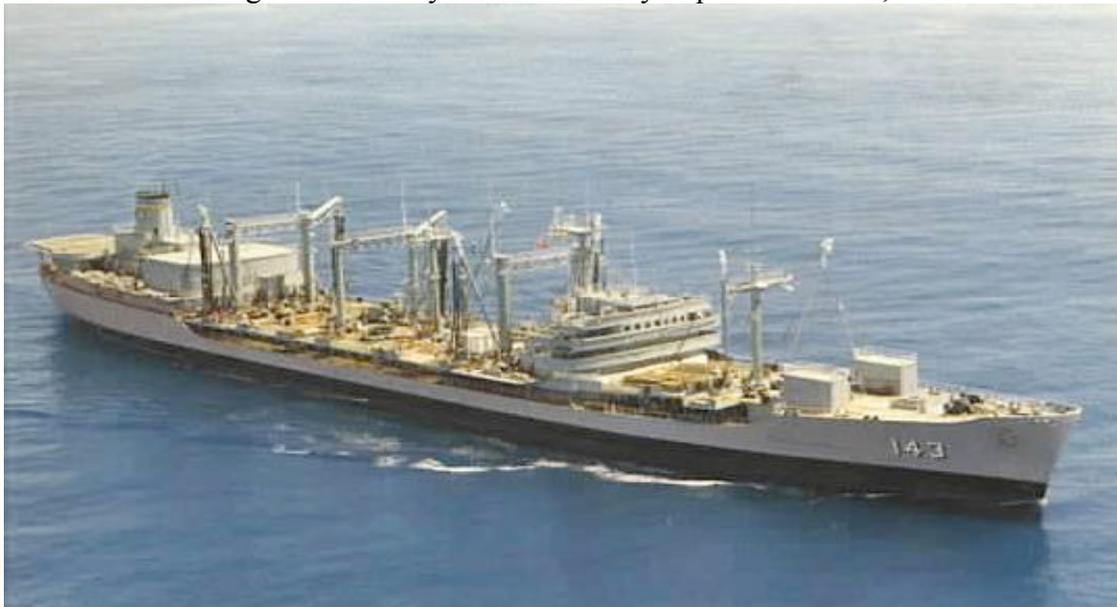
The USS Neosho was the newest class of fleet oilers designed to carry bulk oil, diesel fuel, aviation gasoline and JP-5, fuel for jet aircraft. Longer than two football fields, when fully loaded, the freeboard [distance between the water line and the first deck] was almost twenty feet. With a draft of thirty-six feet, she very seldom pulled along side a
